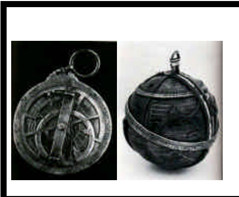
Astrolabes (Left: from the 9 th C; right: 15 th C) were used for measuring the altitude of heavenly bodies above the horizon, and so determining the time of day or night. Readings are taken by means of rotatable alidade, a diametrical rule with sights.
